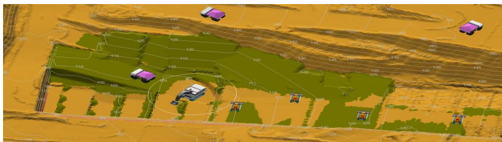
Figure 10. Back stacking and design low wall ramp
