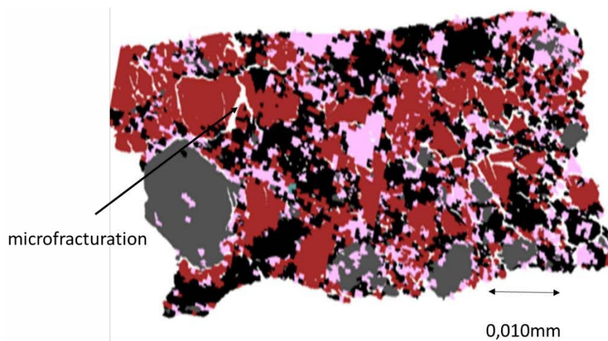
Figure 5. Example of a micro-fractured particle of a HPGR
