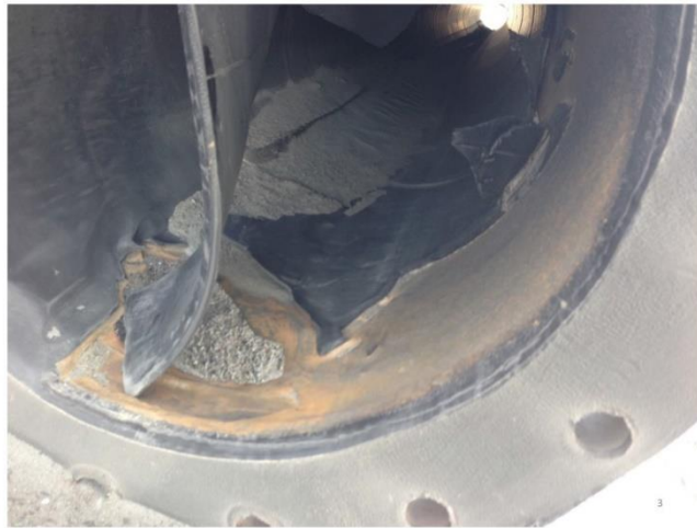
Photo 1. An example of peel off caused by sand and pressure (Dan Chamberland, 2014)
