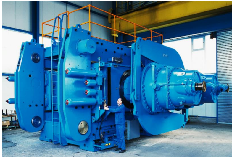
Figure 2. Typical example of a state-of-the-art HPGR
