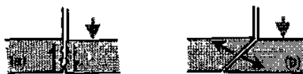
Figure 5 Liner failure modes at small block displacements caused by either shear rupture or diagonal tensile rupture.
