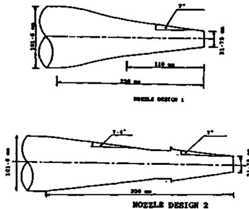
Figure 5. The two nozzle designs
