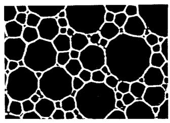
Figure 1. Structure of an emulsion seen through a microscope.
