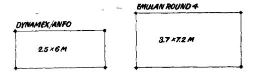
Figure 6. Original and final drillpattern after change of explosive.
