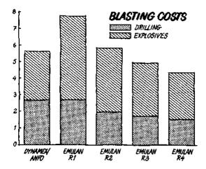
Figure 7. Total blasting cost for different explosive combination.
