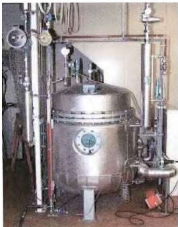
Figure 11. Pressure vessel for ageing in oxygen-enriched water at elevated temperature and pressure.
