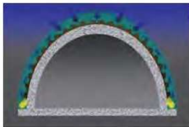
Figure 3. The 'umbrella principle'
