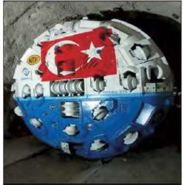
Figure 1. Double Shield TBM used for excavation of Yamanli II HEPP Project 1st Stage Energy Tunnel (Robbins)
