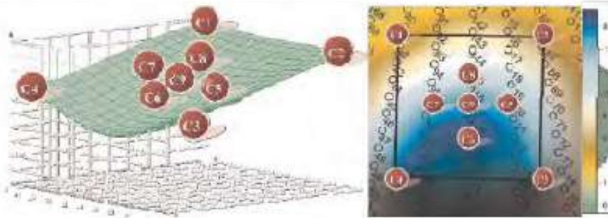
Figure 12. Concurrent grouting simulation: 3D view of the heave measured on plate 2
