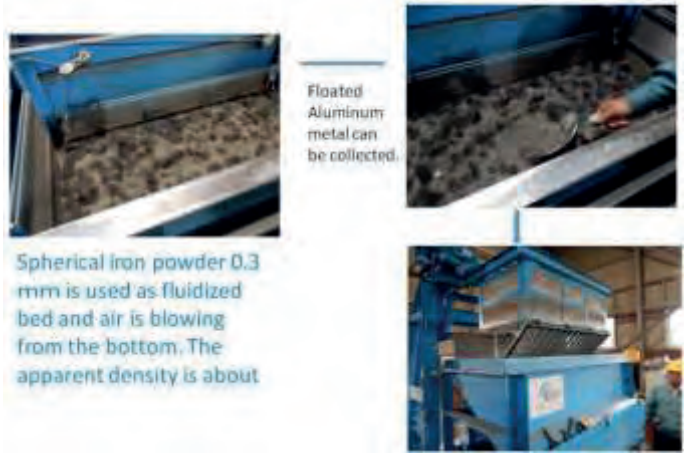
Figure 28. Dry fluidized bed separation using fine iron powder. (Nagata Engineering, 2017)
