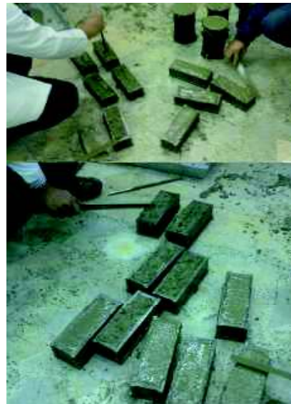
Figure 9. Flexural test specimen preparation
