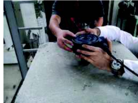
Fig 6. Load cell putting on circular load area
