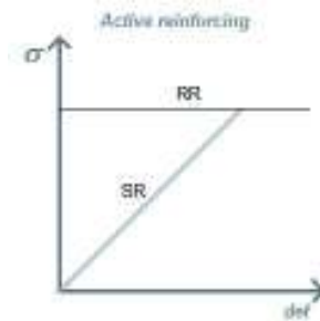
Figure 15. Active reinforcing reaction and support sidewall reaction
