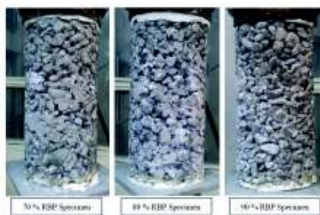
Figure 5. Fabricated model bimrocks with three different rock block proportion (RBP) in cylindrical mould of size 150*300 (mm*mm)
