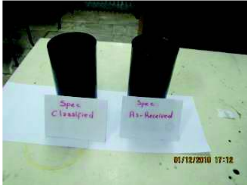
Figure 9. Consolidations of classified and as-received Spec tailings under their self weights in molds (Ercikdi et al., 2013)
