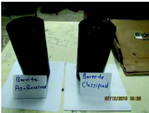
Figure 10. Consolidations of classified and as-received bornite tailings under their self weights in molds (Ercikdi et al., 2013)
