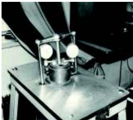
Figure 3. Swelling test in an oedometer under loading
