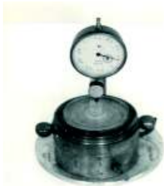
Figure 2. Test of inflation in a free cell oedometer (without piston)
