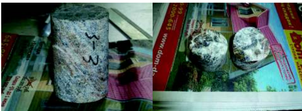
Figure 5. Cylinder specimens of the apatite-nepheline ore before and after destruction
