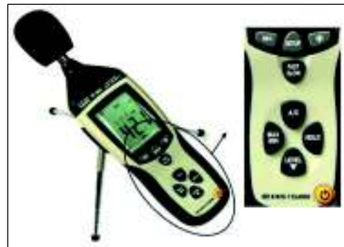
Figure 2. Noise level meter used for the measurements
