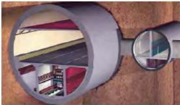
Figure 2. Tunnel profile Silberwald combined road/metro traffic tunnel
