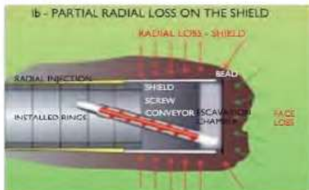
Figure 4. Loss of radial shields
