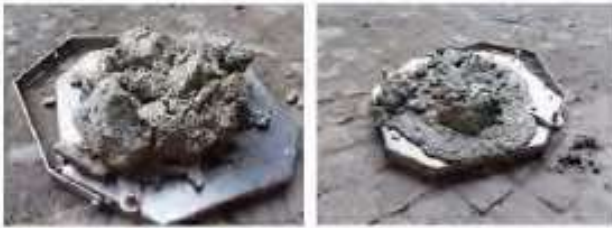
Figure 1. Same sample of soil before and after the addition of foam
