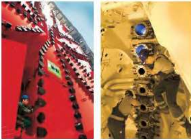
Figure 6. Accessible cutting wheel spokes in free air for tool changes
