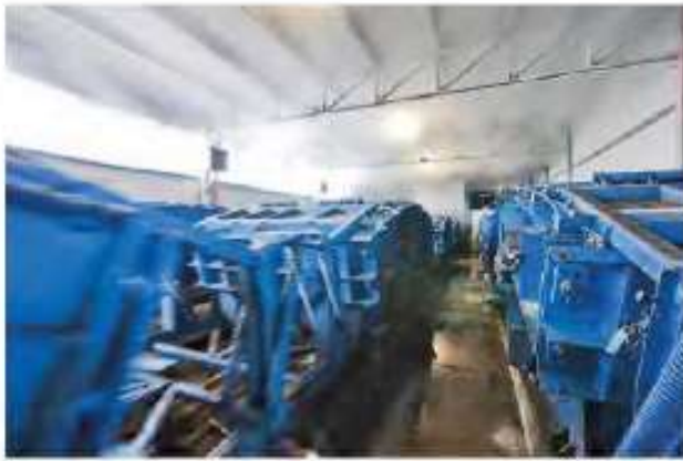
Figure 6. Carousel system with four sets of moulds
