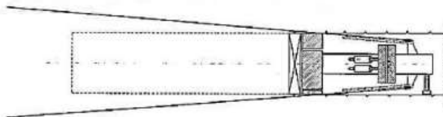
Figure 5. Positioning the drilling equipment for ground investigation or for drilling injection holes with a TBM (Maidl et al., 2008)
