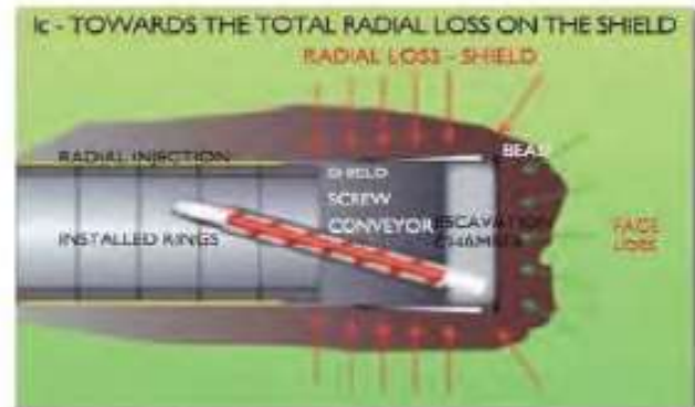
Figure 5. Loss overall radial shields
