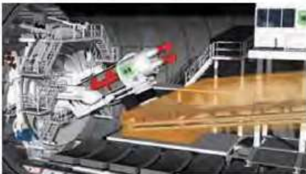
Figure 7. Interface – material handling from the screw conveyor to encapsulated conveyor belt
