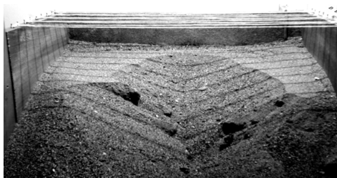
Figure 2. A closer look from front. Settlement occurred. The shadows of the above horizontal ropes which are set every 5 cm (total 8) are clearly visible on the sand. First shadow closest to us is section A, the last shadow section is I.
