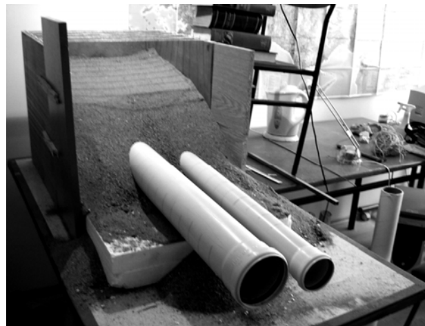
Figure 9. 110 mm and 75 mm diameter tunnels before driven.
