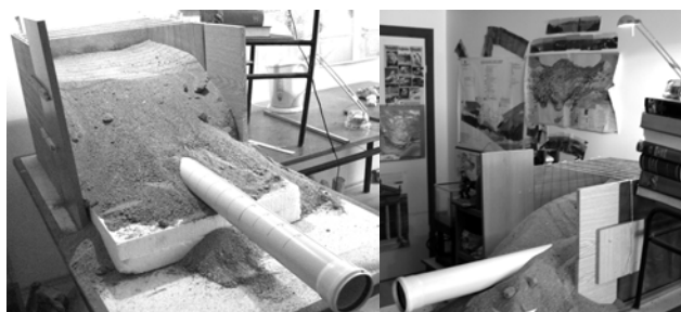
Figure 1. Apparatus used in the experiments. Tunnel (pvc pipe) of 75 mm diameter and overburden thickness of 3.5 D. Light source (upper right corner) used to observe rope shadow in detail.
