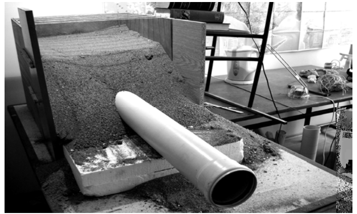
Figure 7. 110 mm diameter (D2) tunnel before driven. Overburden thickness is 154 mm.
