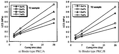
Figure 2 Unconfined compressive strengm versus curing time for the cemented paste backfill samples produced from me tailing T2 using (a) PKC/A binder and (b) PKC/B binder
