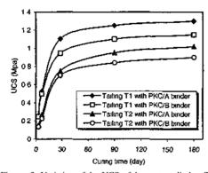
Figure 3 Variation of the UCS of the paste cylinders TI and T2 using 7 wt% binder in the course of curing time
