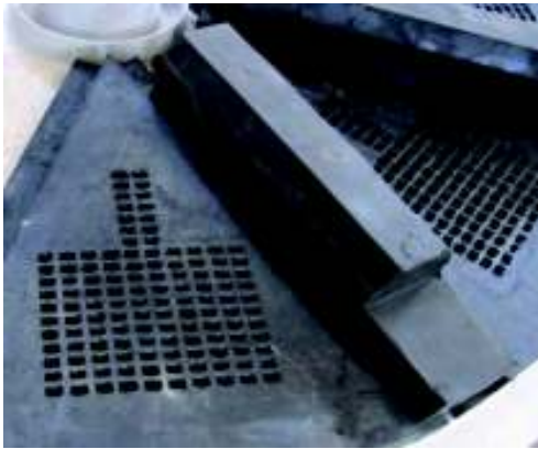
Figure 10. End discharge grate of ball mill of pilot plant of Gol-e-Gohar iron ore processing complex
