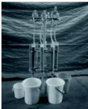
Figure 2. Columns used for leaching tests
