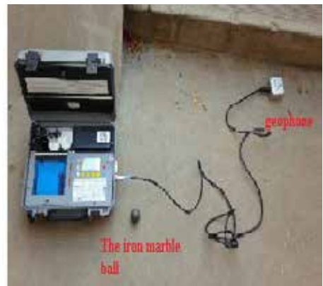
Figure 3. The vibration device and the steel ball used in the tests
