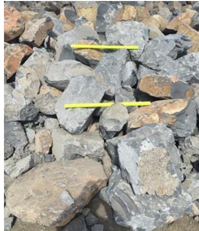
Figure 8. Oversize piled at a separate stockpile. Scale is 1m.
