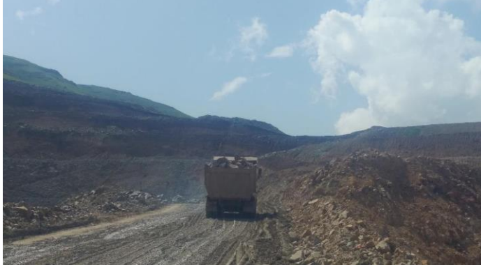
Figure 10. The overloading of a mine truck
