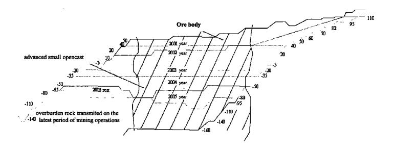
Figure 2. Fonning of advanced small opencast at mining of Sokolovskii opencast.
