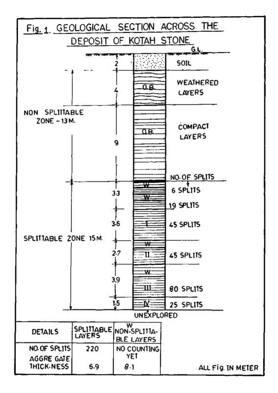
stone layer breaks non-dimensionally depending free face available. It is then sized to largest possible by chiesel and hammer. Finally/ it is splitted along natural slip planes to yield single solid slab ready to use.
