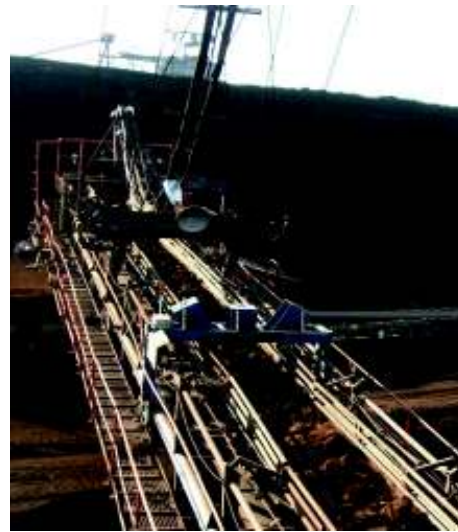
Figure 5. On-belt Ash-analyzer on the discharge boom of a bucket chain excavator
