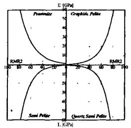
Figure 6. Elastic characteristics of rock masses.
