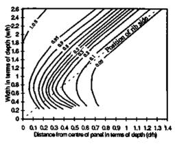
Figure 3 Nomogram for predicting shapes of transverse subsidence profiles for different *w/h* ratios in the Southern coalfield of NSW
