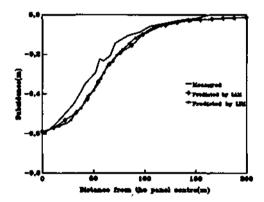
Figure 5 Comparison of the shapes of measured and predicted transverse subsidence profiles for case 2
