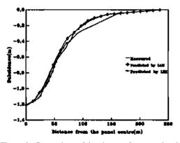
Figure 8 Comparison of the shapes of measured and predicted transverse subsidence profiles for case **4**
