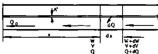
Figure 3. Model for a duct with longitudinal aperture
