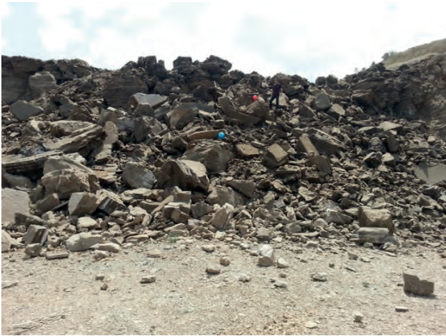
Figure 4. Rock pile of blast round with plaster stemming at Tuncbilek open pit lignite stripping blasting
