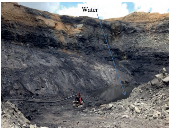
Figure 8. Water on the floor blocking access to the seam
