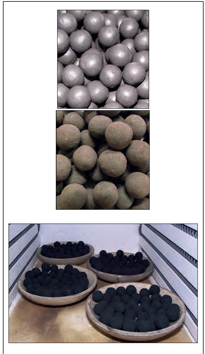
Figure 3. Green and dry pellets and sintering of pellets in the box-furnace.
