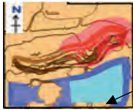
Figure 10: Year1 (in red, the mining sequence, in blue, the waste material dumping sequence)
