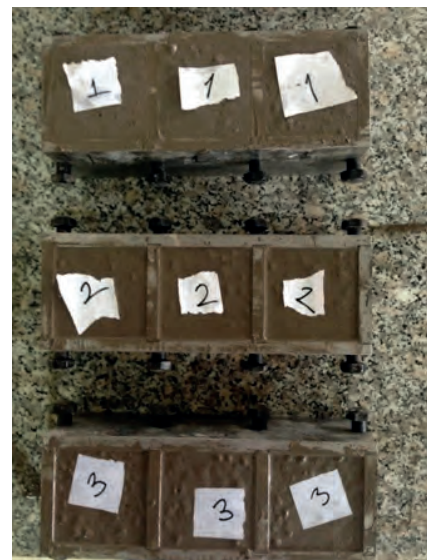
Figure 7. Light-weight concrete mixture to fill the mold.
