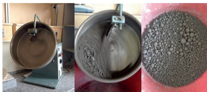
Figure 1. Pelletizer disc and light-weight aggregates.
