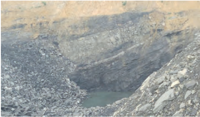
Figure 3. Coal seam crosscut by a fault
