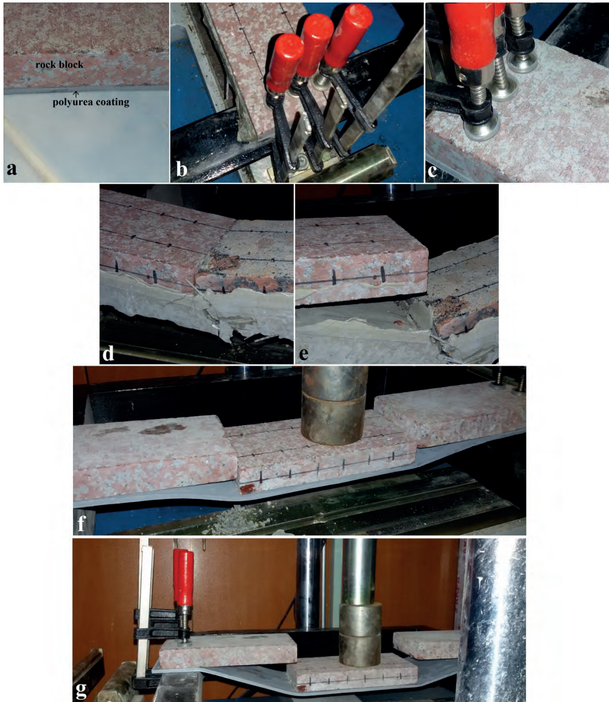
Figure 12. a) Polyurea coating, b and c) fixing concrete and polymer coated blocks, d) cracked concrete liner, e) Separation of concrete adhesion surface, f) a mid block carried by polyurea adhesion surface, g) totally separated polyurea adhesion surface
