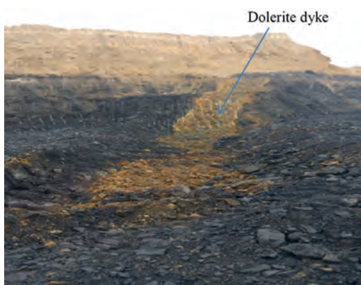
Figure 6. Dolerite dyke that cut through the coal seam
