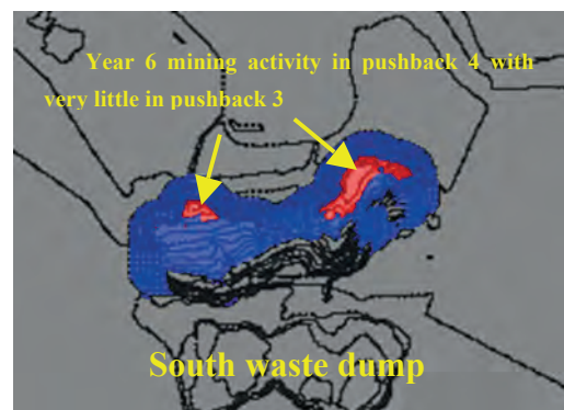
Figure 12: Year 6 of Mashamba schedule graphical sequence, as generated from the NPV software, in red, the mining activity (ore and waste mining), in blue is the topography of the optimized area.
