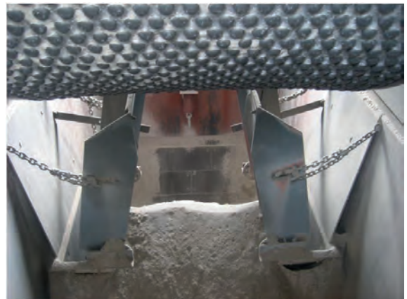
Figure 3. Installation below the rollers to separate the edge and centre products
