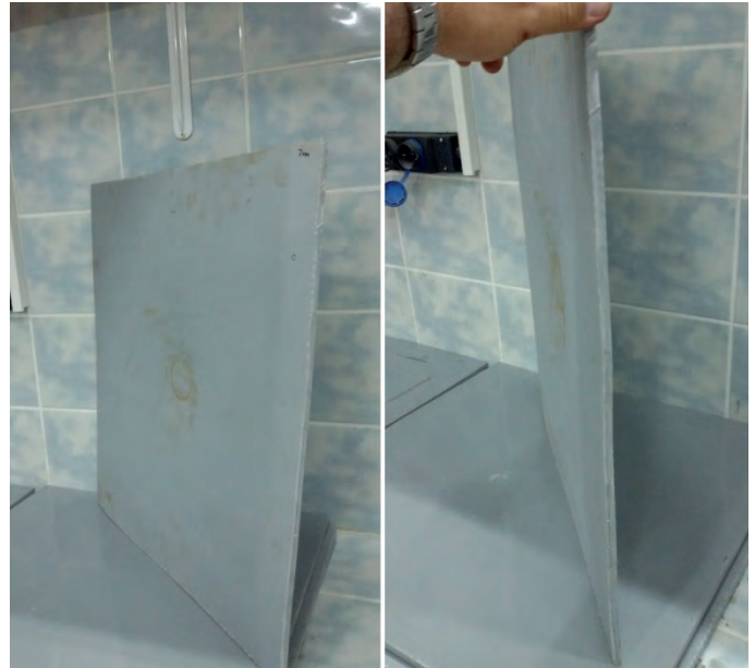
Figure 11. A tested TSL slab loading specimen
