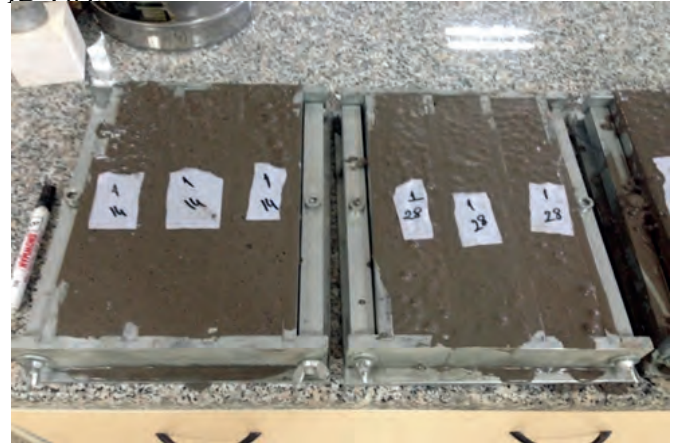
Figure 10. Light-weight concrete mixture to fill the mold.
