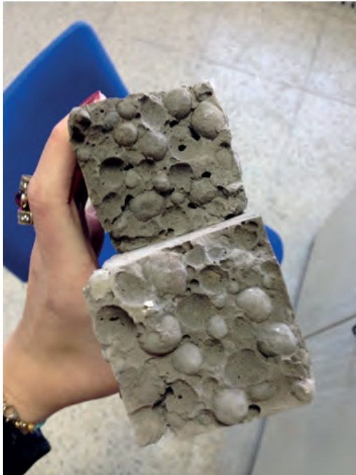
Figure 13. Fracture surface of light-weight concrete samples after flexure strength test.
