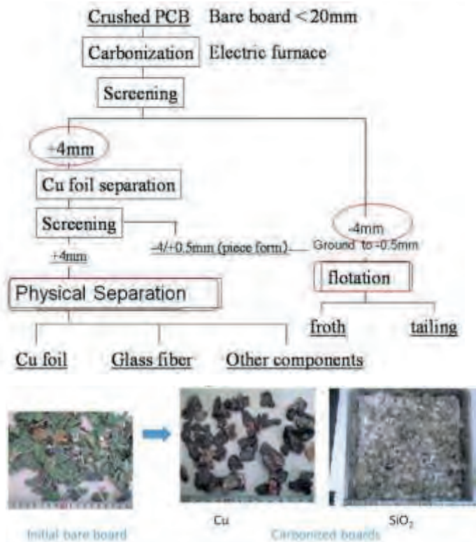
Figure 31. Recycling flowsheet of printed circuit board by physical separation and heat treatment and photos of separated copper and silica by carbonization. (Fujita, 2014)
