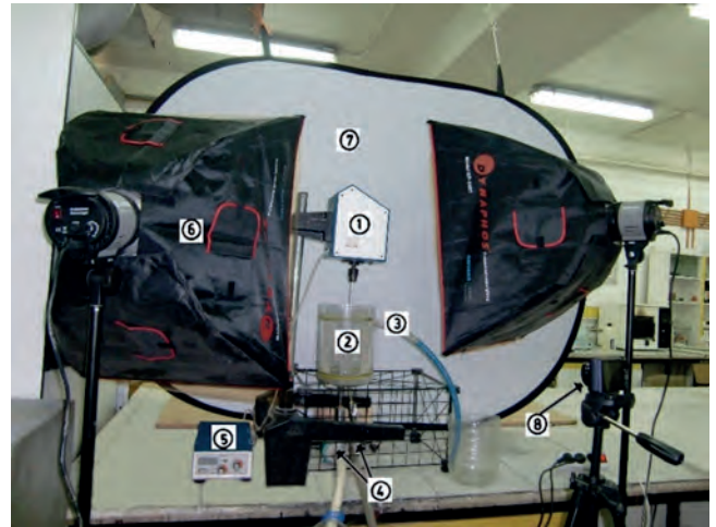
Fig. 2. Experimental equipments (1-mixer motor 2-mixer vessel 3-outlet 4-aqueous and organic inlets 5-impeller speed controller 6-projectors 7-reflecting surface 8-camera)
