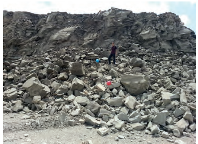
Figure 3. Rock pile of blast round with drill cuttings stemming at Tuncbilek open pit lignite
