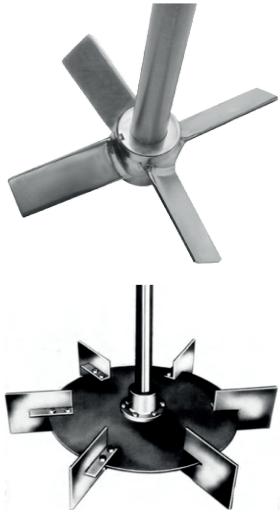
Figure 1. Traditional axial flow 45° pitched blade turbine (top) and radial flow Rushton turbine (bottom) (Oldshue, 1983)
