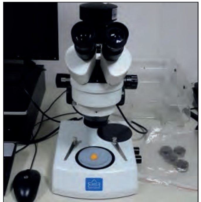
Figure 2. Stereomicroscope for getting sample photos.
