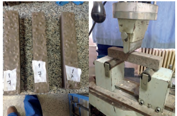
Figure 11. Putting the samples into the press machine.
