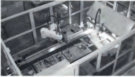
Color sorter to separate copper metals 95% grade at 0.2t/hr
