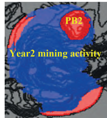
Figure 29: Year 2 of KOV pit accelerated schedule graphical sequence, as generated from the NPV software, in red, the mining activity (ore and waste mining), in blue is the topography of the optimized area. PB for pushback 2.
