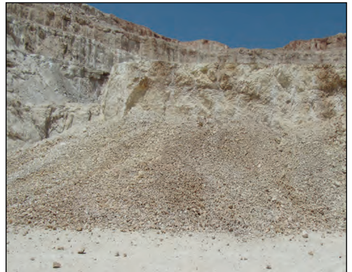
Figure 6 Electronic blast muckpile
