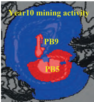
Figure 23: Year 10 of KOV pit schedule graphical sequence, as generated from the NPV software, in red, the mining activity (ore and waste mining), in blue is the topography of the optimized area. PB for pushback 5 and 9.
