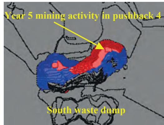
Figure 11: Year 5 of Mashamba schedule graphical sequence, as generated from the NPV software, in red, the mining activity (ore and waste mining), in blue is the topography of the optimized area.
