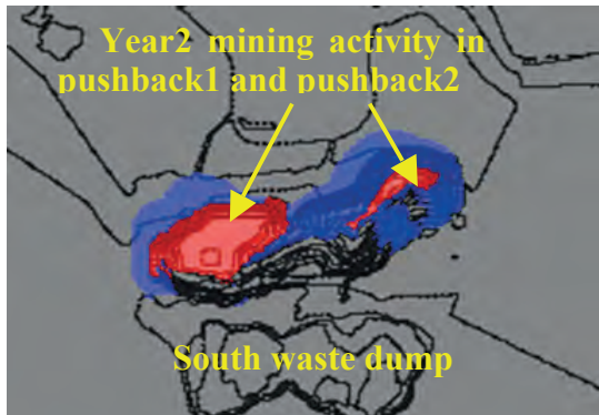
Figure 8: Year 2 of Mashamba schedule graphical sequence, as generated from the NPV software, in red, the mining activity (ore and waste mining), in blue is the topography of the optimized area.
