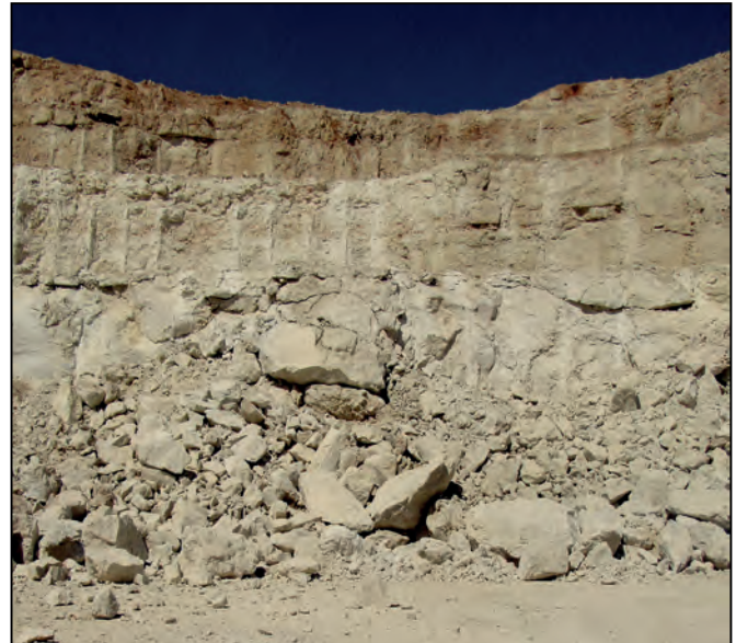
Figure 5. Nonel poor fragmentation and toe problem
