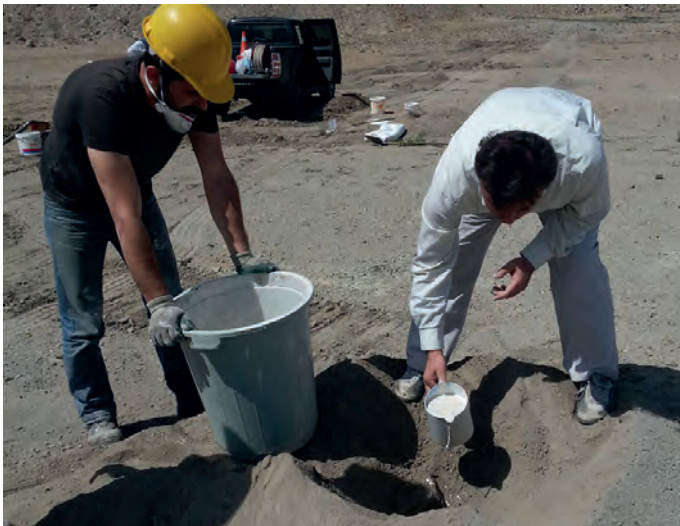
Figure 1. Application of plaster paste to hole collar at Tuncbilek open pit
