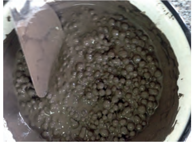
Figure 6. The mixture of fly ash, cement and lightweight aggregate.
