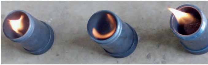
Figure 9. Briquettes combusting inside the steel cylinders.
