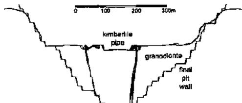
Figure 1 Cross-section of the final pit design
