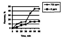
Figure 3. Kinetics of gold cementation recovery for "non-vibrating" bed cementator. Initial concentration of solutions - 8 and 700 ppm, flow rate 20 ml/min
