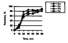
Figure 5 Influence of foreign ions addition on gold cementation with "vibrating" bed cementator. Initial concentration of solutions, ppm Au -123, Cu - 215, Pb 87 2, Fe -70 Solution flow rate 20 ml/min. Shaking frequency f=53 Hz, amplitude A= 4 mm
