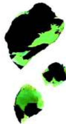
Figure 4. Separation of tungsten ore using XRT analysis. Black areas represent tungsten compounds.
