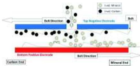
Figure 2. Detail of separation zone
