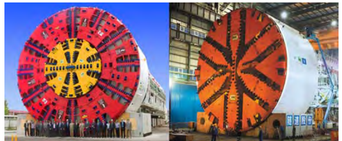
Figure 1. Trend towards increasing diameters: EPB-shield (Spain, 2005) Ø 15,20 m and Mixshield (China, 2006) Ø 15,43 m (Pictures: Herrenknecht AG)
