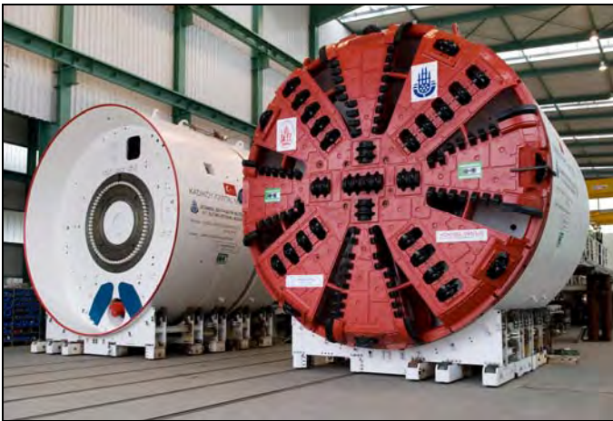
Figure 7. EPBM for the Istanbul Metro, Kadiköy - Lot 1.
