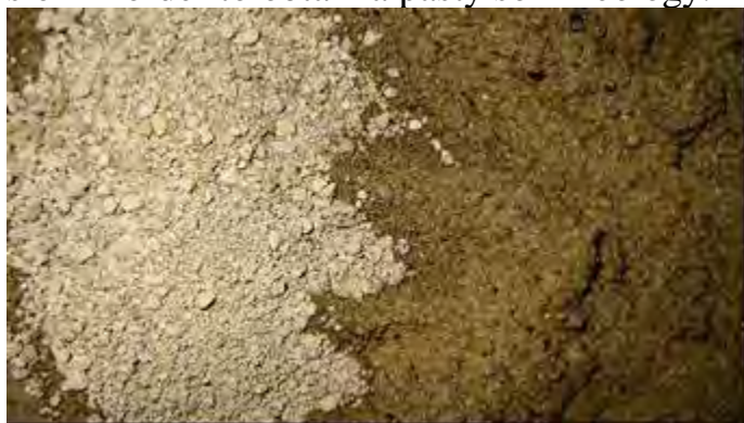
Figure 5. Comparison of original pure dry porous soil and homogeneous paste after mixing with foam and polymer
