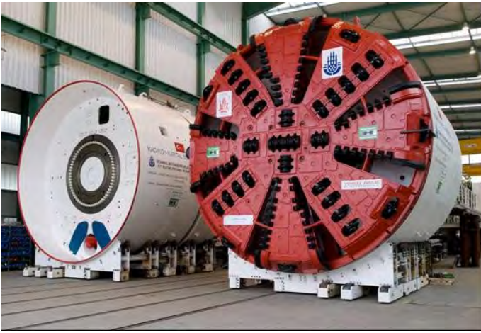
Figure 2. General view of the TBMs in the factory for Kozyatağı-Kadıköy Metro Tunnels
