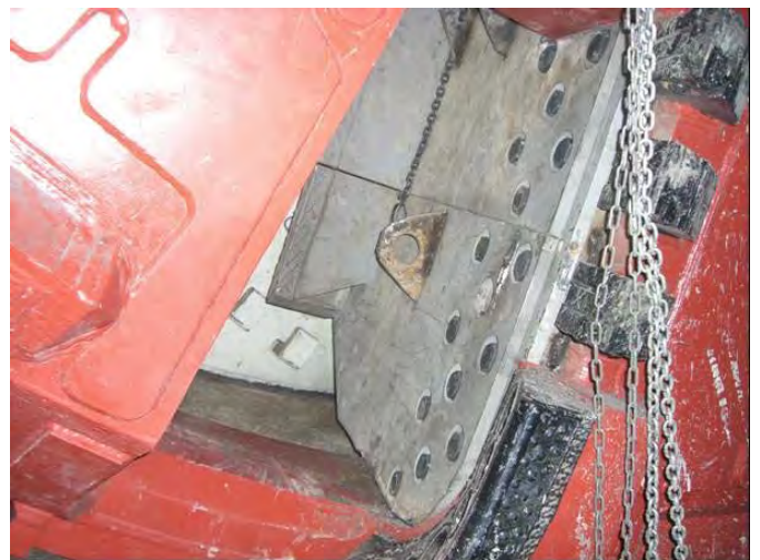
Figure 13. Buckets that were assembled on the cutterhead
