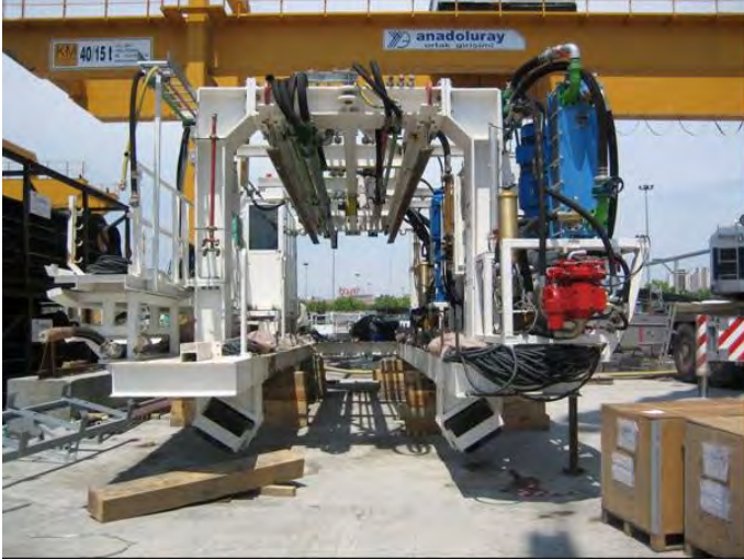
Figure 6. Gantry 1 with the hydraulic equipment, boogies assembled and supported with wooden blocks
