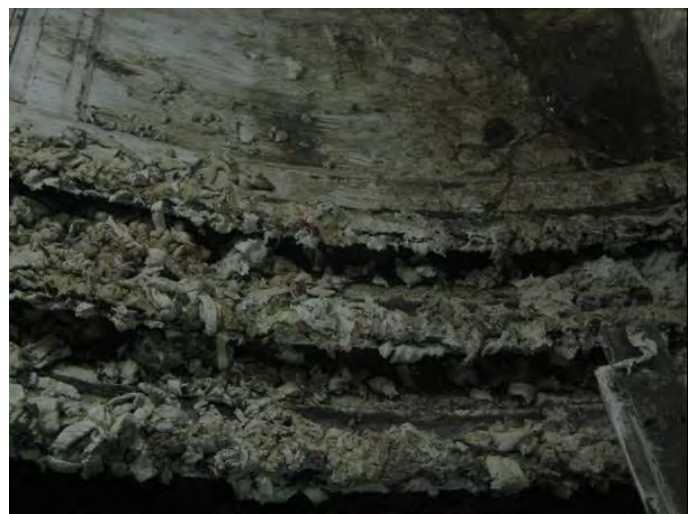
Figure 15. Grease on tailskin brushes
