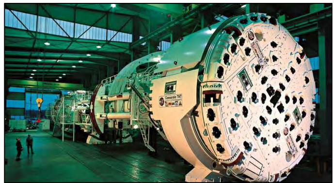
Figure 3. Single Gripper-TBM for the Gotthard Base Tunnel in Switzerland.
