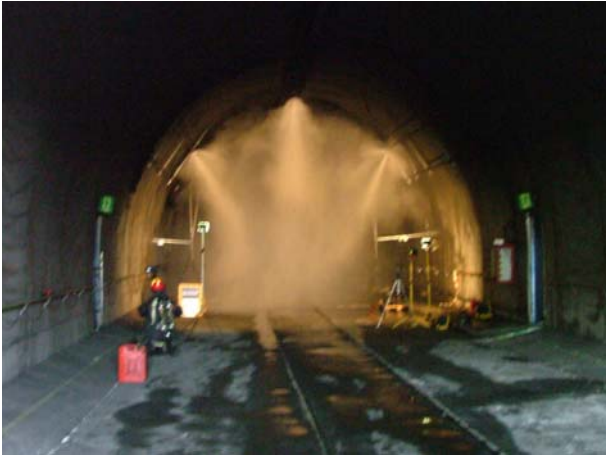
Figure 4. Test of a water mist system (Fogtec), conducted within the UPTUN Research Project.
