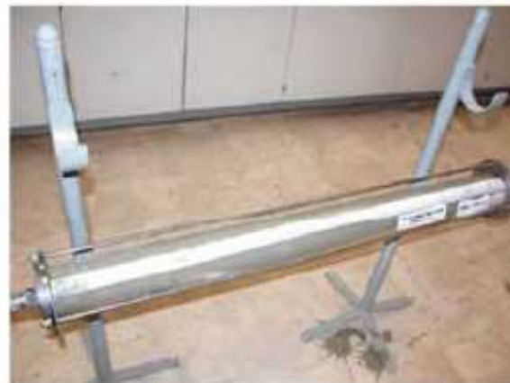
Figure 8. Injection test with Ultrafine 12
