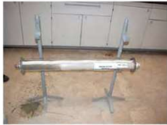
Figure 6. Injection test with Ultrafine 20
