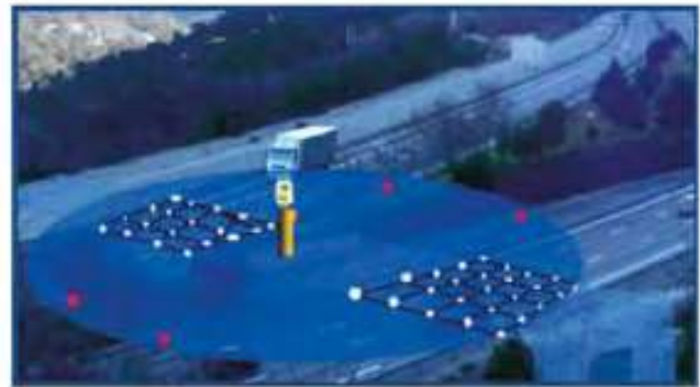
Figure 11. Artificial network of measuring points to control settlements of the roads above the tunnel construction
