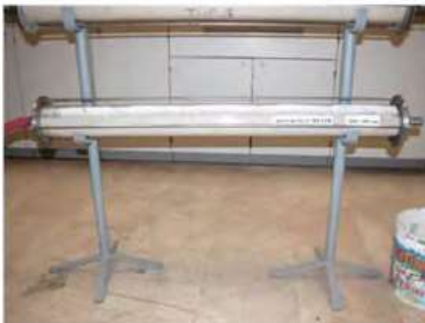
Figure 5. Injection test with CEMI 42.5R
