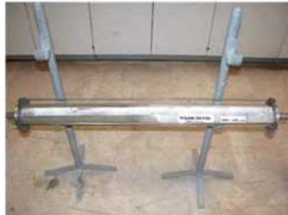
Figure 7. Injection test with Ultrafine 16
