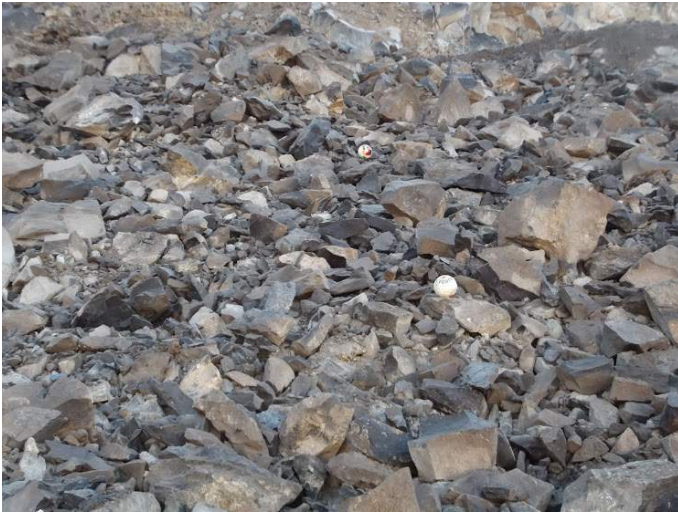
Figure 4. Rock pile from blast round with plaster stemming at Asagi Caglayan Basalt quarry
