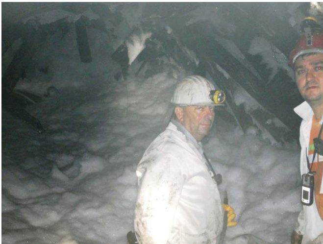
Figure 8. Result of phase B: The head gates Kalin Damar and Taşlı Damar are totally inundated with foam (in front: ventilation engineer and assistant)
