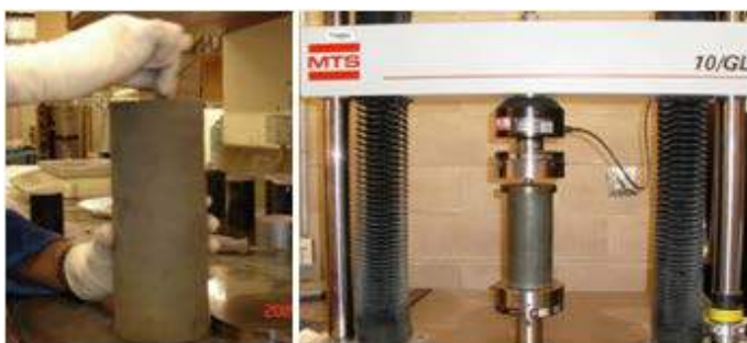
Figure 7. Photos of (a) a sample rectification and (B) CPB samples under MTS Sintech 10/GL mechanical press
