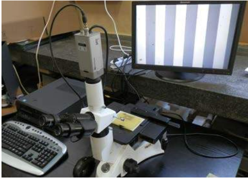
Figure 7. The installation for the analysis of the deposition plates, on screen appears a snapshot of a detail of the deposition plate obtained at 100x.
