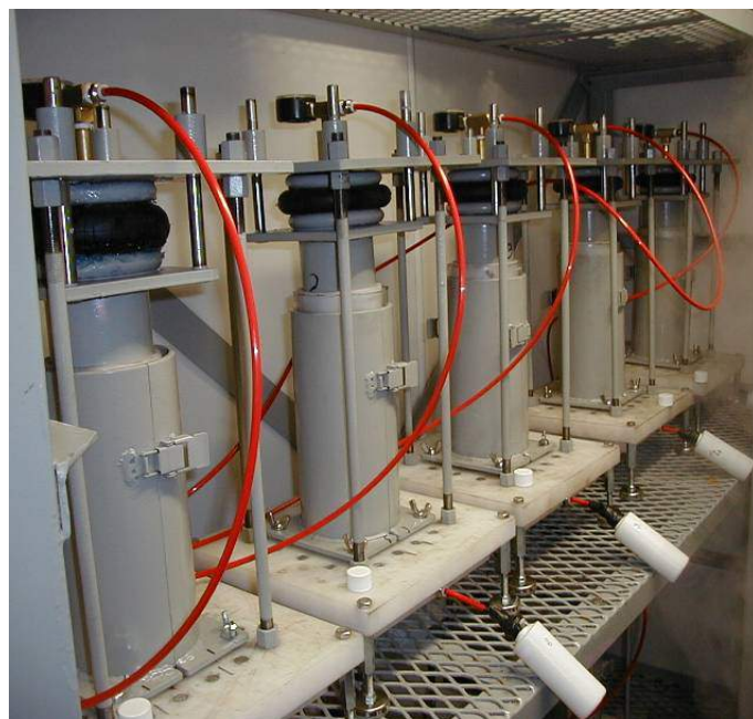
Figure 2. Photo showing the backfill samples cured within the CUAPS apparatus
