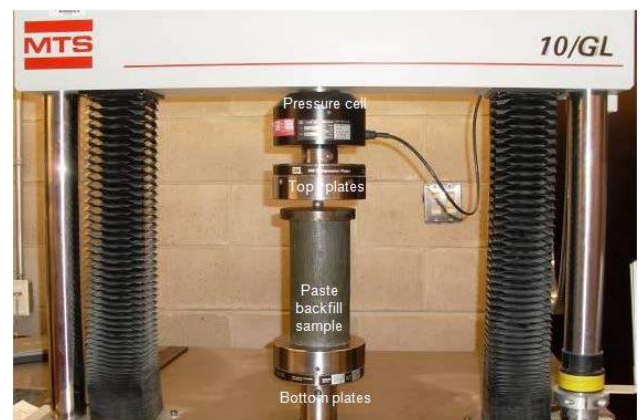
Figure 6. CPB sample subjected to UCS test
