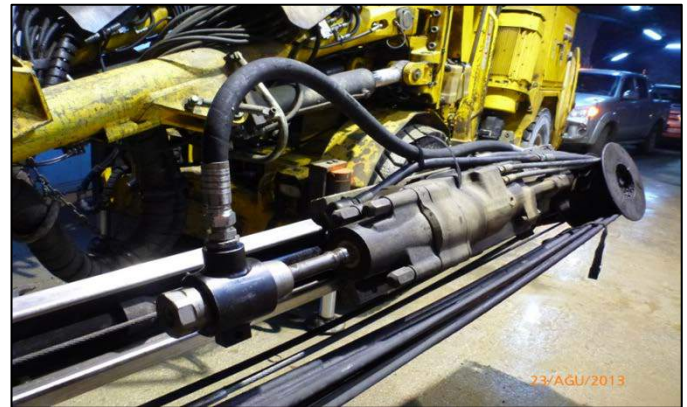
Figure 8. Adapter attached to jumbo drill and connected to a grouting pump that sends grout into bolts while drilling.
