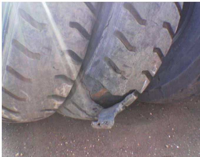
Figure 3. The tread separation
