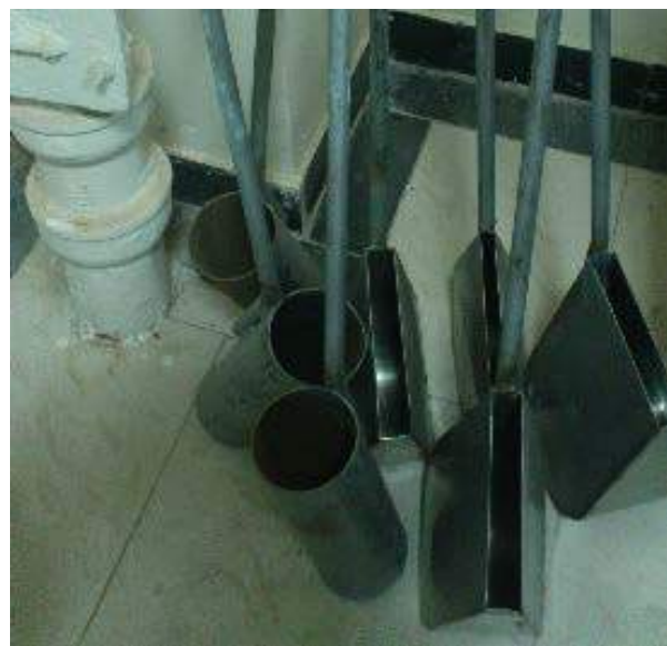
Figure 2. Sampling cutters for collecting samples from the secondary flotation circuit
