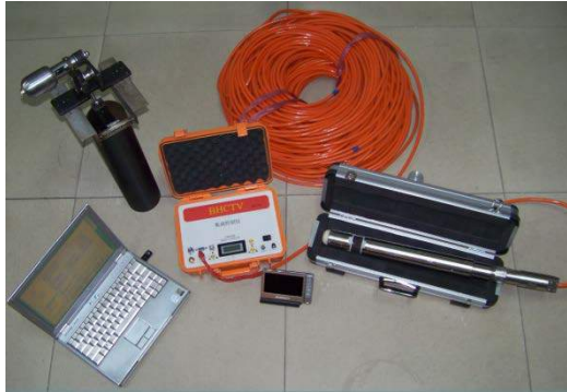
Figure 1. Digital panoramic borehole camera system
