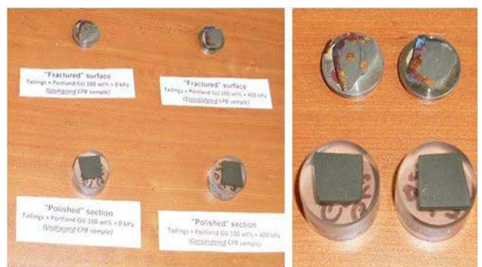
Figure 5. Photos of polished and fractured paste backfill samples.
