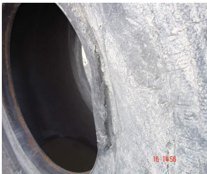
Figure 5. The toe damage
