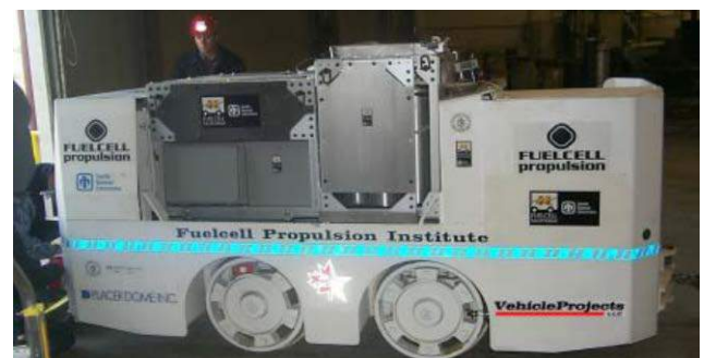
Figure 2. Underground mining locomotive adapted to be fuel cell powered (4 ton -7.2 kW).
