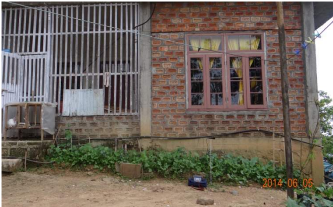
Plate 4. View of vibration monitoring point near the foundation of an adjoining residential house at Ch: +400 m blasting location
