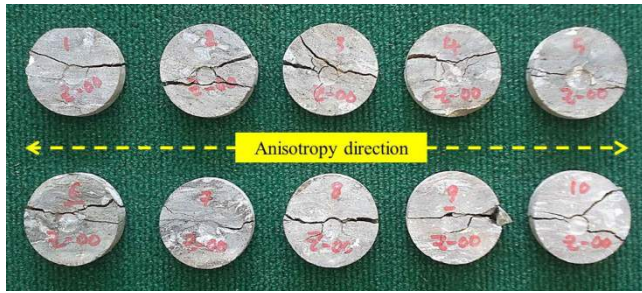
Figure 4. Crack propagation parallel to anisotropy directions at \beta=0^\circ
