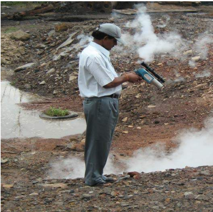
Figure 2. Thermal investigation using Heat spy Infra-red Thermometer near Giddi Sub-station and Mining workshop, CCL.
