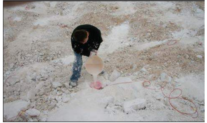
Figure 1. Application of plaster paste to hole collar
