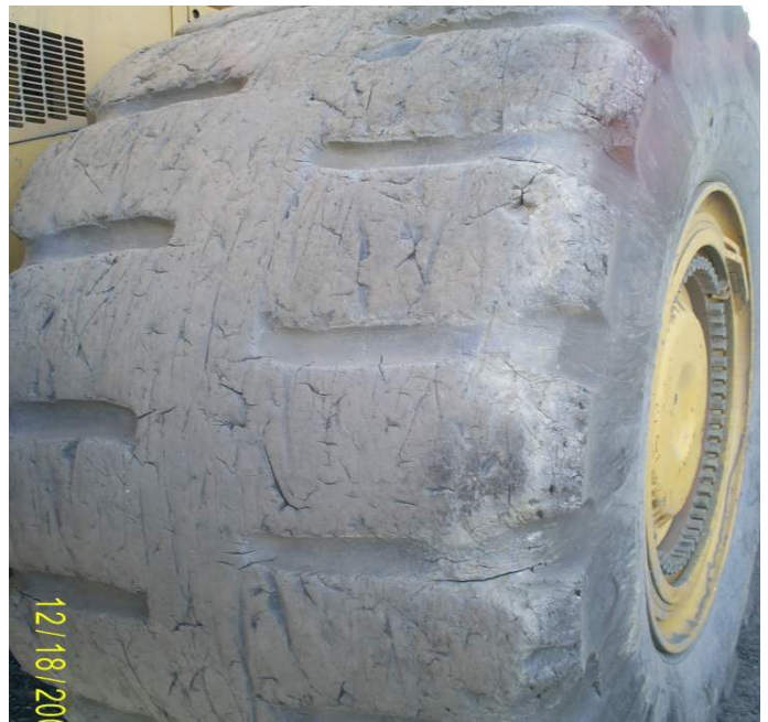
Figure 2. The tire wear
