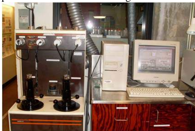
Figure 8. Micromeritics Autopore III Model 9420 mercury intrusion porosimetry
