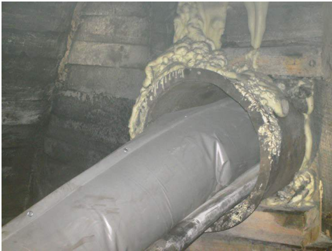
Figure 7. Auxiliary ventilation through the head gate dam Kalin Damar, the smaller foaming hose (DN 75) is also visible
