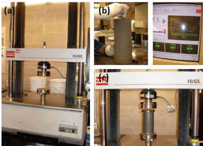
Figure 3. Photos of (a) MTS Sintech 10/GL mechanical press, (b) a sample rectification with typical results, and (c) the CPB sample under compression testing.
