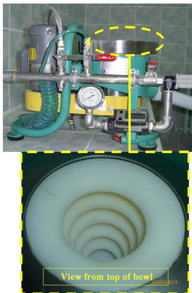
Figure 4. A photograph of Knelson Concentrator used in experiments
