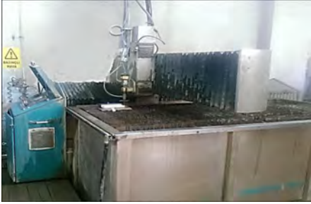
Figure 3. The AWJ used in the study.
