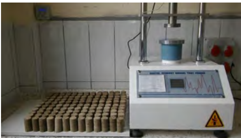
Figure 2. Digital unconfined compressive device and samples
