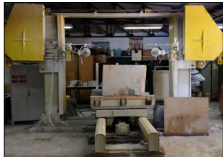
Figure 1. General view of the mono-wire block cutting machine.
