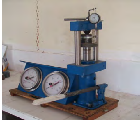
Figure 3. The Indentation testing using point load apparatus.
