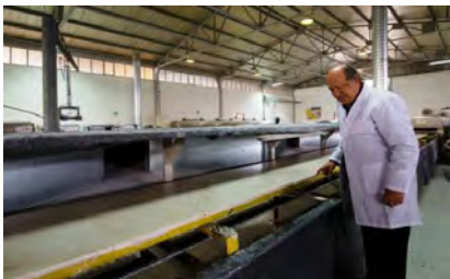
Figure 5. Epoxy treatment line at Soylu marble plant
