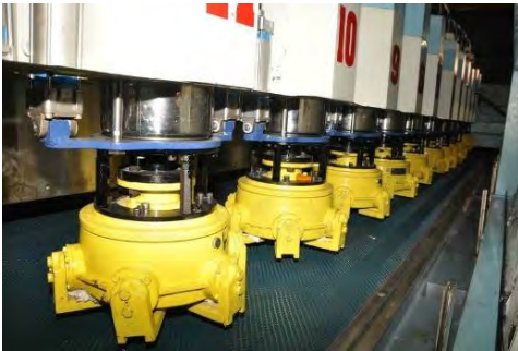
Figure 9. Typical multiple head polishing machine used by the ornamental stone industry. (Source: Carosio & Paspaliaris, 2003).
