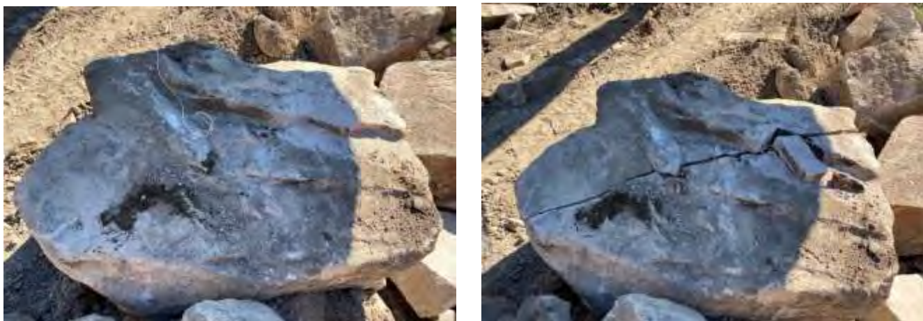
Figure 5. Splitting of a boulder with one charge of 0,050 kg. Mixture #1 in single blasthole with length 0,60 m.
