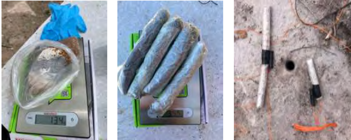
Figure 6. Propellant based cartridges with Mixture #3 in plastic foil bag
