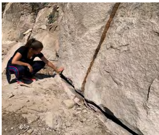
Figure 4: Effect of single crack after experimental blasting with propellant-based non-detonating compositions (Mixtures #2 and #3).
