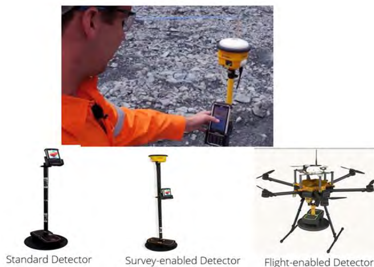
Figure 10. Locating BMMs in the blast pattern (pre-blast) and muck pile (post-blast).
