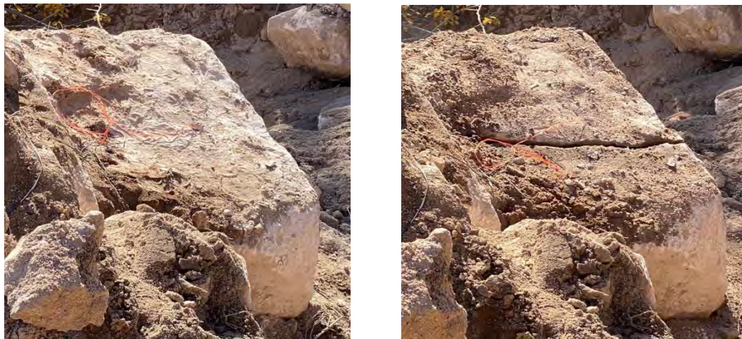
Figure 2: Effect of rock-splitting with chain charges with petards with Mixture #1
