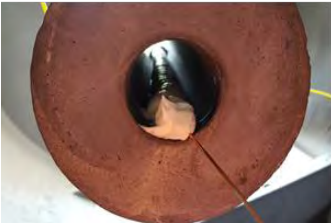
Figure 3. Decoupled string emulsion Ø22 mm in Ø50 hole and a VoD probe in a mortar confinement (Nyberg et. all, 2017).
