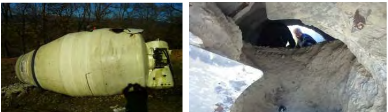
Figure 9. Concrete mixer – exterior and interior with consolidated concrete inside
