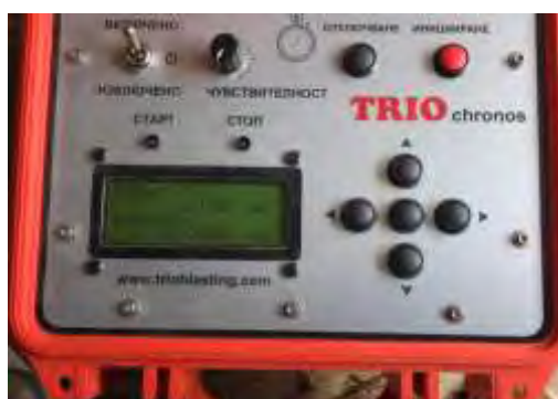
Figure 3. Apparatus for measurement of VOD optical sensors
