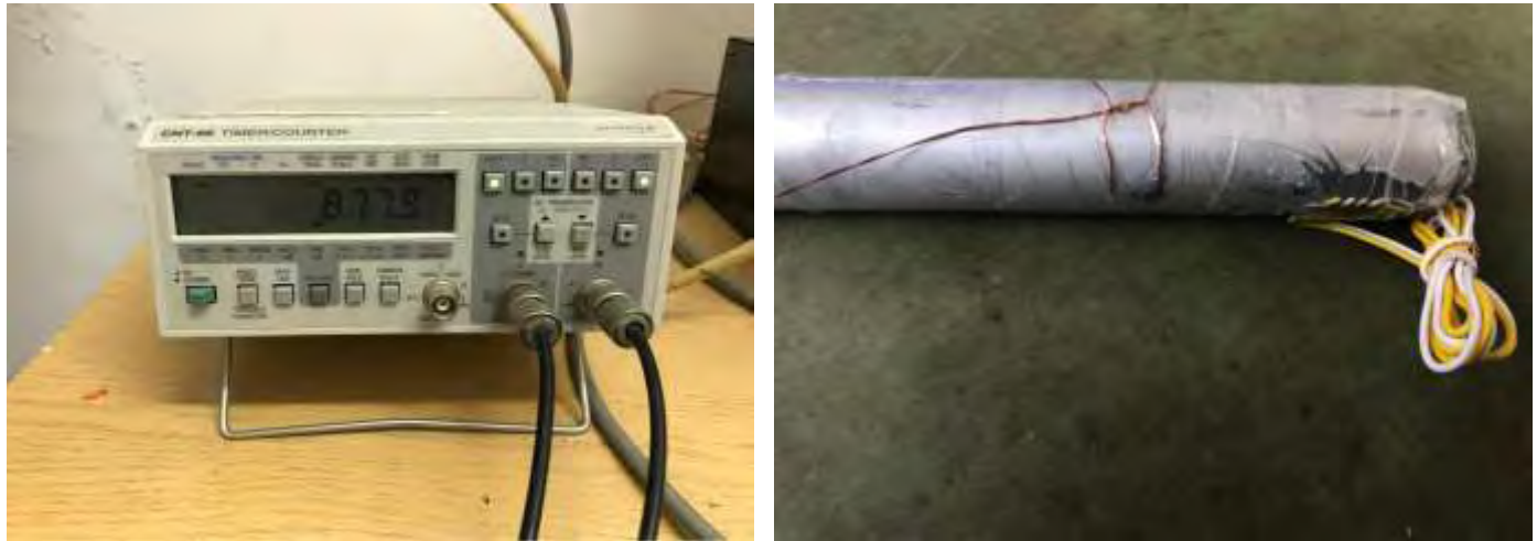
Figure 4. Apparatus for measurement of VOD and sample with impact sensor.
