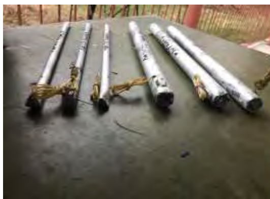
Figure 2. Loaded and plugged aluminium pipes with electric igniter - ready for test samples
