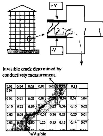
Figure 9. Monitoring of the cracks on concrete blocks.
