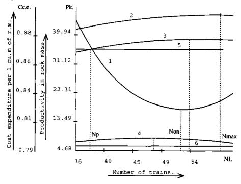
Graph-analytical method of defining the optimum amount of stocks circulating in the pit transport system. 1-4 are graphical dependeces corresponingly: according to specific expenditures, according to the rock mass, according to the opened mass, according to ore; 5,6 - plan indices of the overboding mass and ore.  $N_p$ , N« , Nmx - accordingly rational, optimal and maximum possible amount of locomotive compounds.
