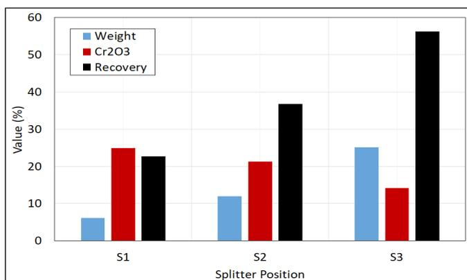
**Figure 4.** Effect of splitter position on concentrate weight, Cr<sub>2</sub>O<sub>3</sub> grade and recovery
