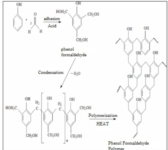
**Figure 1.** Phenol formaldehyde condensation reaction (Frihart, 2005, Özlısoylu 2016).
