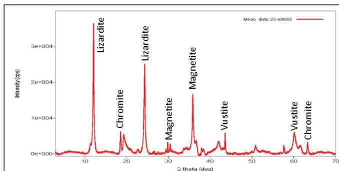
**Figure 1.** X-ray diffraction pattern of the tailing
