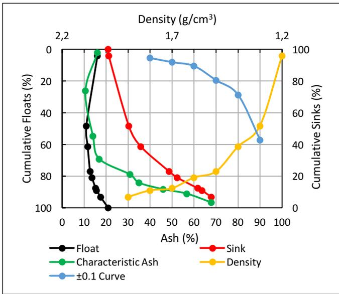
Figure 3. Float-Sink test results for the coarse particles
