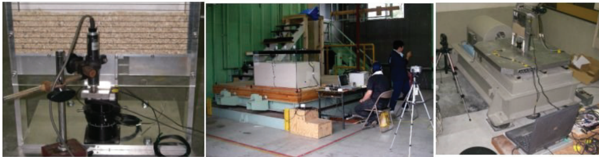
(a) Trap-door experiment (b) tunnel in liquefiable ground (c) dry cohesive medium Figure 5: Views of experiments on model tunnels under different ground conditions
