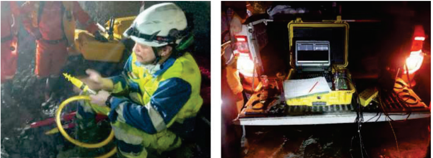
Figure 4. Left: TSP receiver assembly by field geophysicist, right: TSP recording unit
