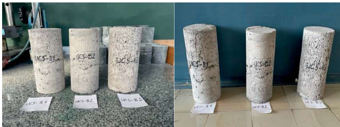
Figure 4. Static deformability test configuration, before and after test
