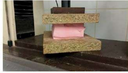
Compression aproximatly 50% of deformation
