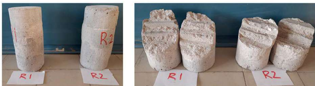
Figure 9: Before test and after test images of concrete samples with rough discontinuity planes
