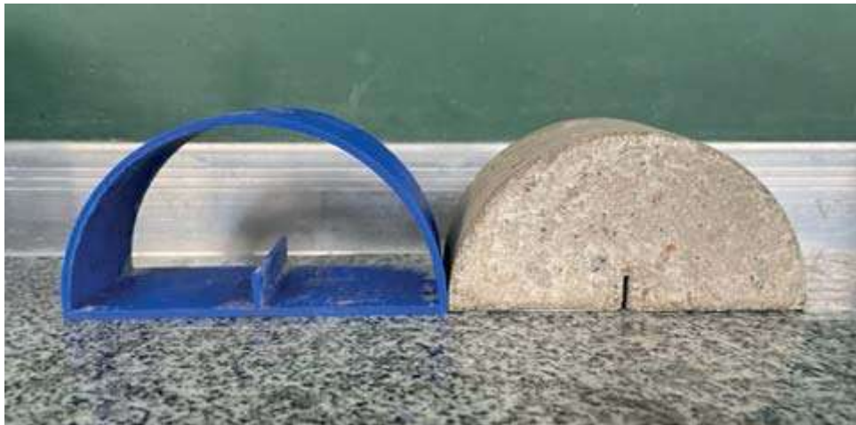
Figure 3. 3D mold of SCB and SCB sample
