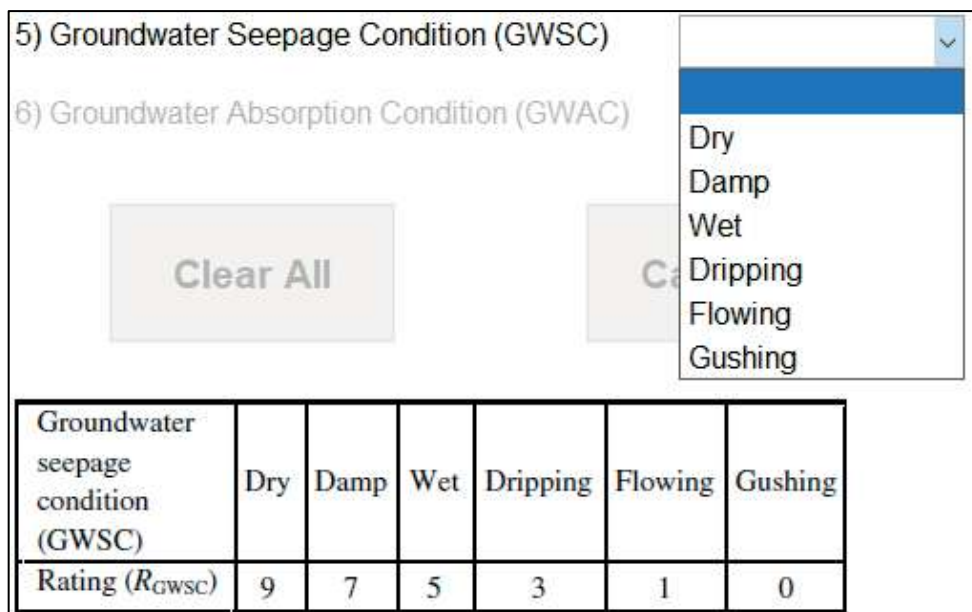
Figure 9. Groundwater seepage condition (GWSC) and R_{GWSC}
