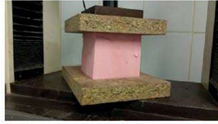
Compression aproximatly 10% of deformation
