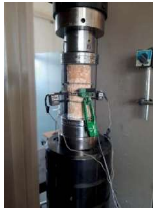
Figure 1: MTS 815 test system and an experiment which conducted static deformability test
