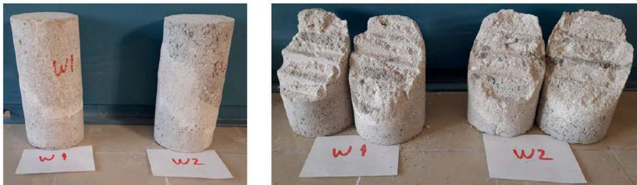
Figure 10: Before test and after test images of concrete samples with wavy discontinuity planes
