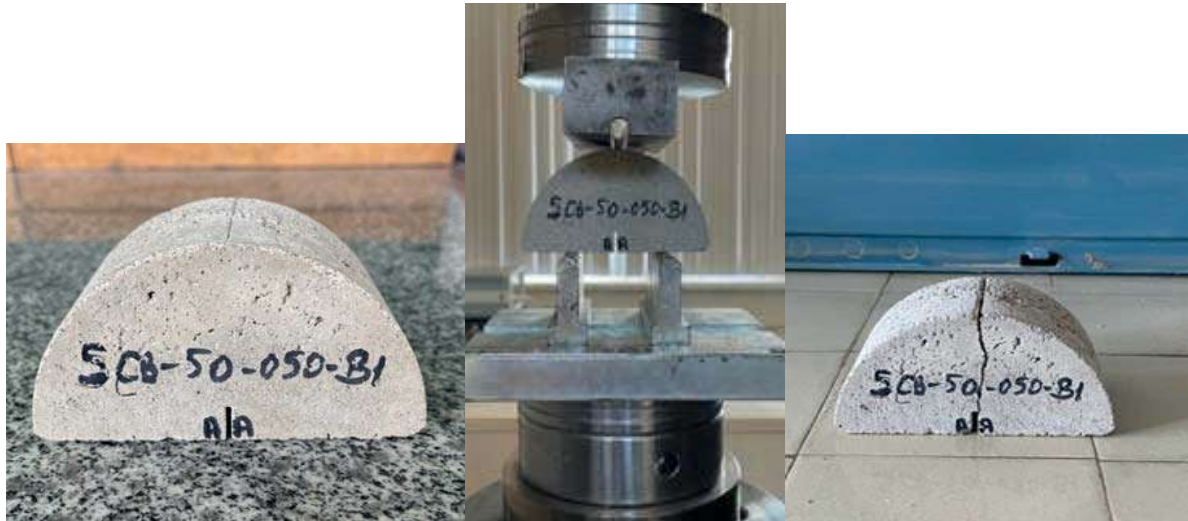
Figure 5. SCB sample before, during and after the test
