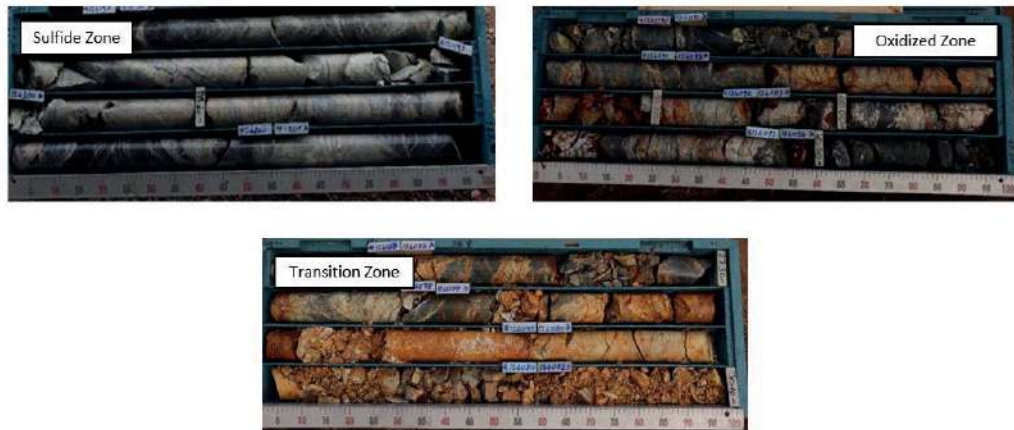
Figure 2. Drill cores taken from the zones
