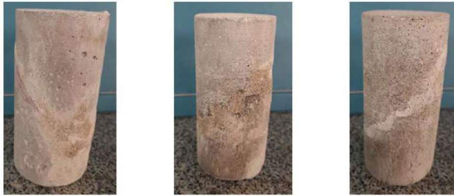
Figure 5: Concrete samples with smooth, rough, and wavy discontinuity planes joined with plaster, respectively
